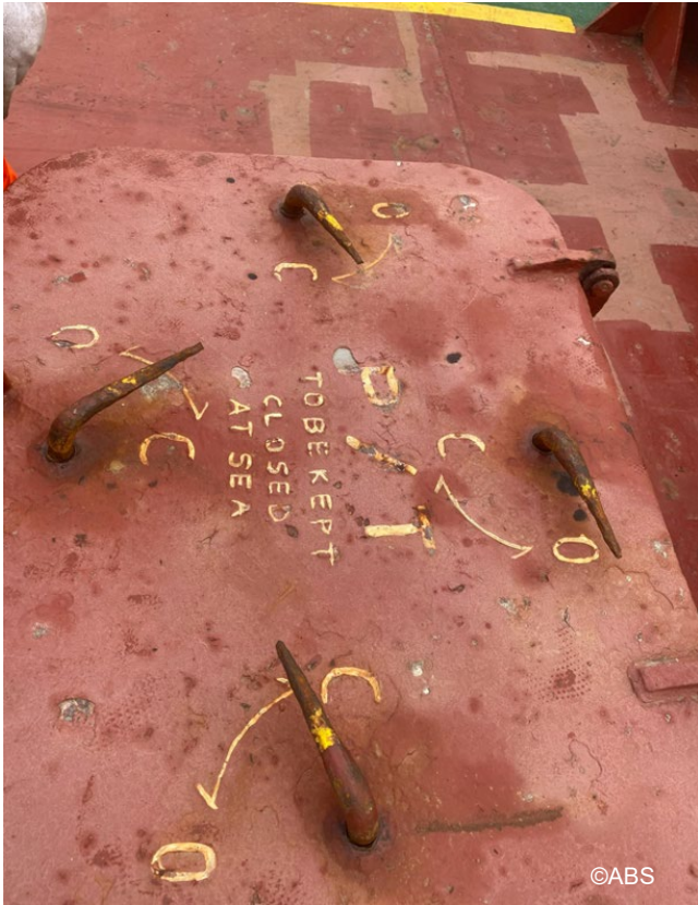
Cargo holds entrance unable to close due to worn handle, turning to 360 degrees on actual closing
